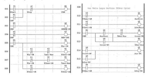
**Figure 7:** The resulting PLC Ladder-logic program generated using TECO-SG2 client software. The PLC uses only 2 inputs, 7 outputs, 1 momentary relay, and 5 timer relays to regulate the process.
